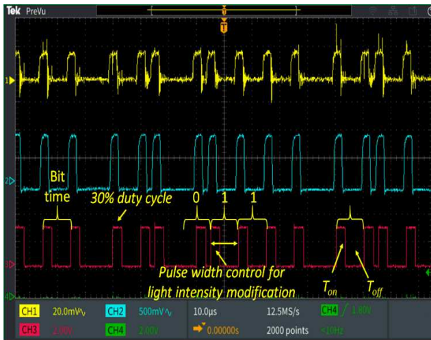
Fig. 3. Oscilloscope print-screen showing the VLC receiver signal processing mode for a 30% duty cycle modulated frame: Channel 1 illustrates the output of the transimpedance circuit; Channel 2 shows the amplified signal; Channel 3 represents the Schmitt trigger output signal used for data processing.
