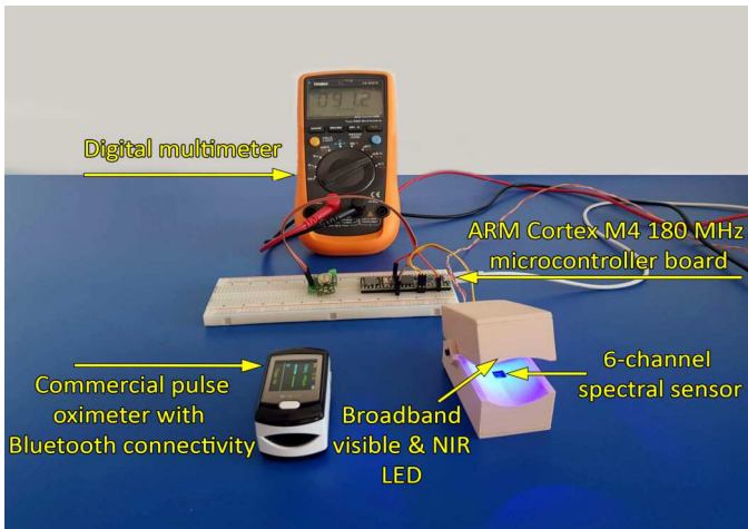
Fig. 5. Developed prototype and its testing setup.
