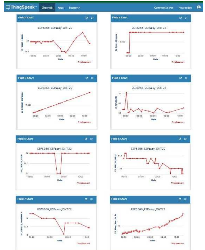
Fig. 9. ThingSpeak example of charts with data from sensors; for a free account, a maximum of 8 charts is offered.
