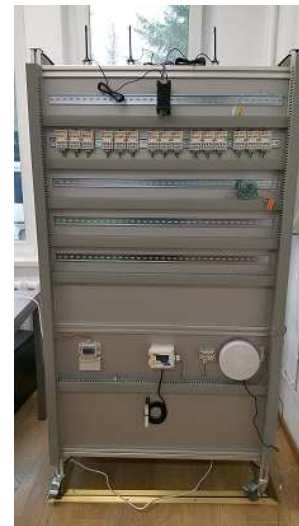
Fig. 4. Testbench with different environmental sensors that will be tested in the LV/MV distribution cells.
