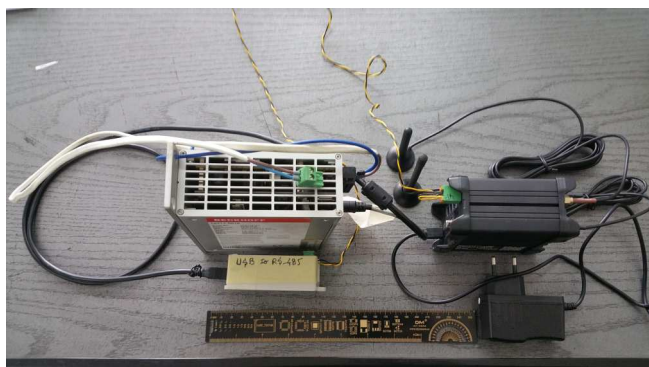
Fig. 13. Practical implementation of ModBus sensors simulation using Node-RED on an industrial PC with Intel Atom, 4GB RAM and OS Win7-64b.
