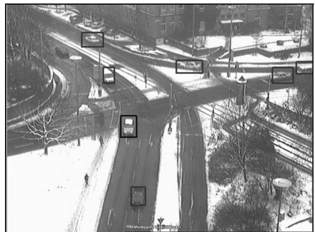
Figure 3. Temporarily undetected moving target (with pixels too close to the background's color)
